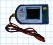
Voltage Sensor is used to measure the electric potential difference at both end of the electric component, it can also measure the voltage of DC and low voltage AC.
